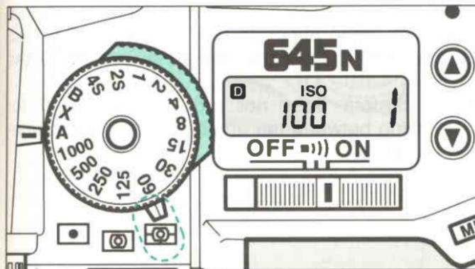
In the multi(6)-segment metering mode, the metering system automatically measures light in six different zones, enabling proper exposure value in a wide variety of normal and adverse lighting conditions.
