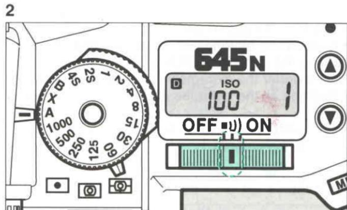
2. With the main switch set to [ ON ], an audible PCV signal is heard when the subject comes into focus.
