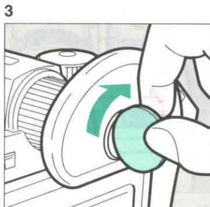
Two types of eyecups, a standard and a larger one are provided as accessories; they may be utilized according to a given situation. The larger is constructed of rubber and designed to fit close to the face for easy shooting.
