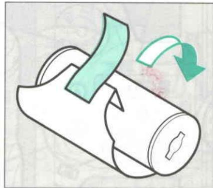
1. After the last frame of the roll is exposed, the camera will automatically wind the film and stops winding as soon as the back of the leader paper is wound to the take-up spool. [End] on the LCD panel is displayed.
