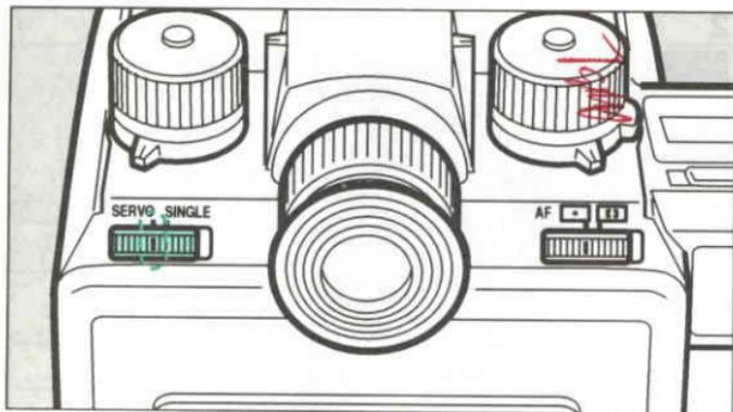
If the shutter release button is held at the halfway position, the lens focuses continuously to follow the subject. The shutter can be released even if the subject is out of focus.
