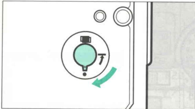
4. Return the multi-exposure switch to the original position to cancel the multi-exposure mode.
