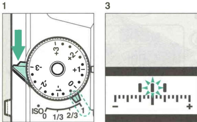
When you take a picture that requires the exposure compensation and it may be difficult to obtain the correct exposure, use this mode to make three different bracketed exposures with different exposure levels. The exposure can be bracketed in 1/3EV, 2/3EV or 1EV steps.
