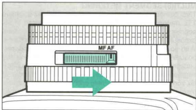
With the Pentax 645 FA lens attached, the lens automatically focuses when you press the shutter release button halfway down.
