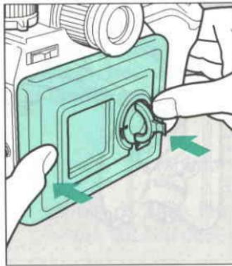
5. Wind the leader paper to the take-up spool until arrow marking on the leader paper aligns with the holder's start mark S and the red line.
