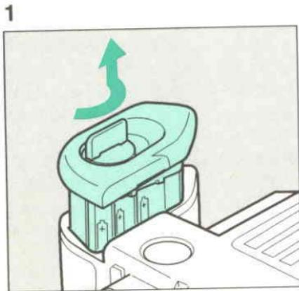
1. To remove the battery holder, lift up the battery holder release knob and turn it in the direction of the arrow.
