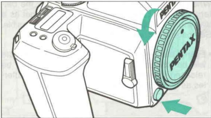
1. Remove the body mount cap while depressing the lens unlock button.
