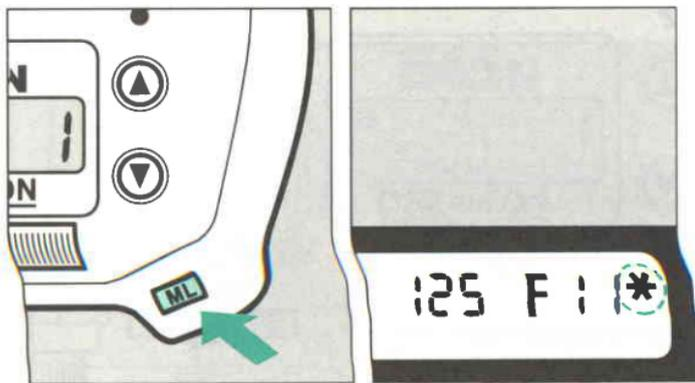
The memory lock function enables an exposure level to be memorized before shooting. The memory lock function is very effective when used along with spot metering. Use the memory lock function to get a correct exposure when the subject occupies only a small part of the viewfinder.
