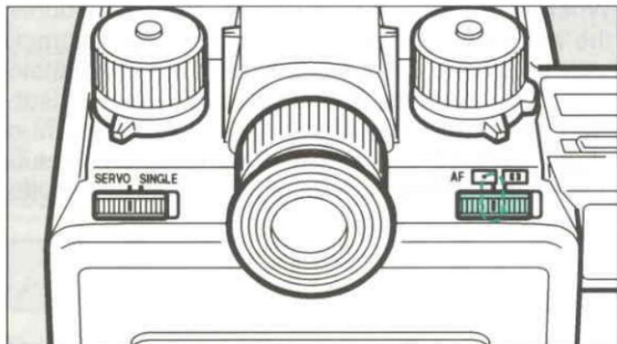
Select the Spot AF Mode to critically focus on a specific spot of the subject which is in the spot AF autofocus frame.
