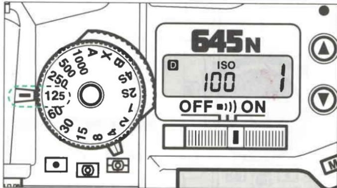
2. Set the shutter speed dial to the desired shutter speed.
