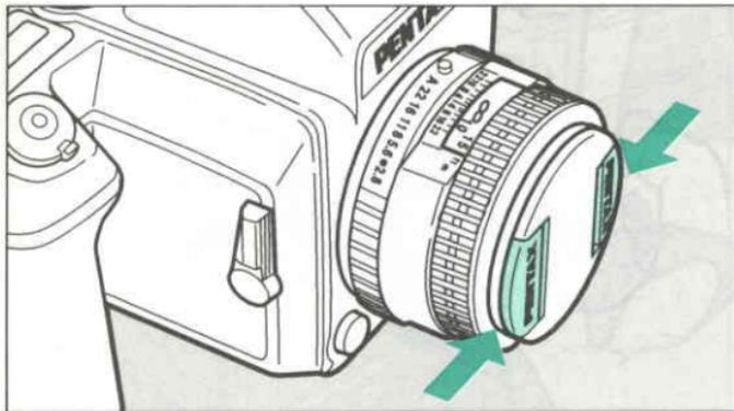
**3. To remove the front lens cap, squeeze the tabs on both sides in the direction of the arrow.**
