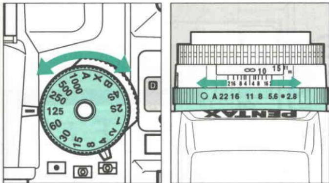
3. Turn either the shutter dial or lens aperture ring until a single bar is displayed in the center of the bar graph.
