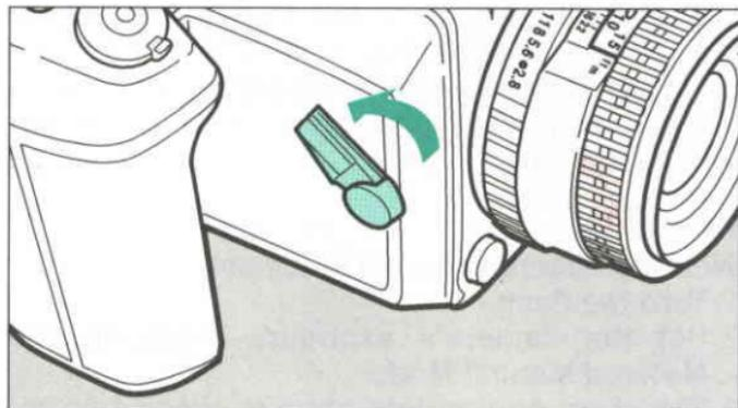
**2. Depress the preview lever. The aperture will stop down to the preset value, and the depth-of-field can be confirmed through the viewfinder.**
