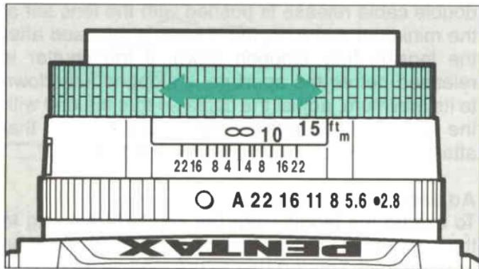
When infrared film and an "R2" or "O2" filter are used, the focal point is different from that of ordinary film exposed in visible light. The autofocus system cannot compensate for this difference automatically.
