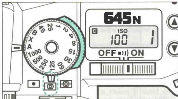
The Spot metering or center weighted metering mode can also be selected in this camera. Select the desired metering mode with the metering mode selector.
