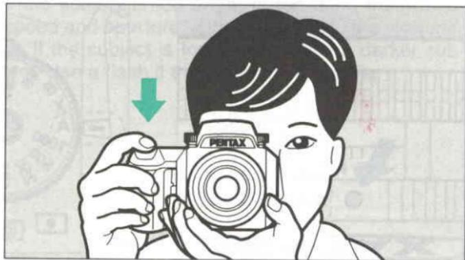
5. Recompose the frame, and depress the shutter release button to shoot the second shot.
