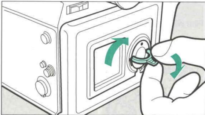
**3. Turn the film holder knob 90° to the right. After attaching the film holder to the camera, fold the film holder knob into its original position.**
